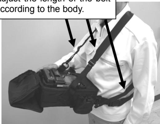
Connect each belt on each hook, put the fusion splicer, and fix with metal fittings.
