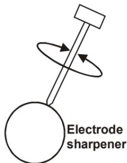
a) Firmly stick the tip of an electrode (approx. 0.5 – 1.0 mm) into the electrode sharpener and turn/twist the electrode 3-4 times.
