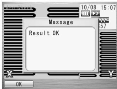
5. When NG, repeat the arc check to determine that the new values are acceptable. It is necessary to remove the fibers and prepare them again with a new cleave. If unsatisfactory results are obtained after 5 – 4 arc check attempts, inspect the electrodes for wear or damage, and replace them if necessary.
