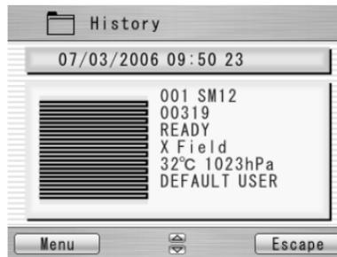
3. Press Menu key and the pop-up shows available functions. Select desired function and press Enter to initiate the operation.
