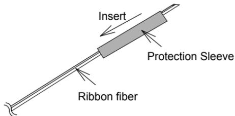
2. Place the ribbon fiber to the fiber holder in such a manner that the ribbon fiber tracers are in the same direction. In this case, set the length so that the ribbon fiber end projects about 30 mm from the holder.
